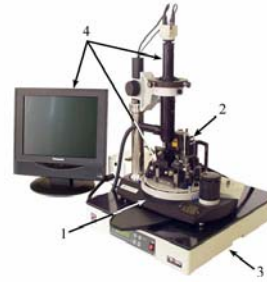
Fig. 2. Atomic Force Microscope NTEGRA Probe NanoLaboratory: 1 – base unit; 2 – measuring head; 3 – vibration isolation system; 4 – optical viewing system.
