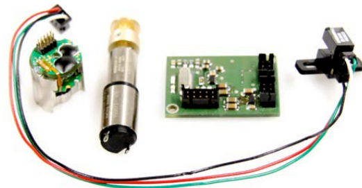
Fig. 8. Motor controller with modular encoder
