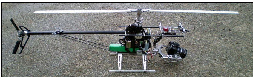
Fig. 10. Remotely piloted platform with 3-axis prototype gimbal
