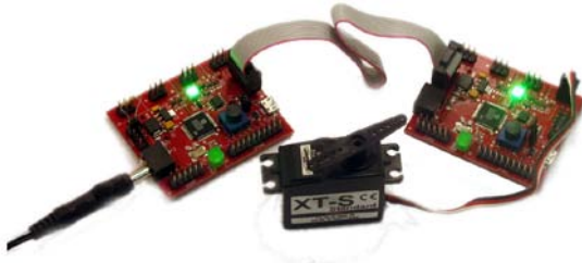
Fig. 5. HomeLab ARM-CAN Kit controller boards connected over the CAN interface
