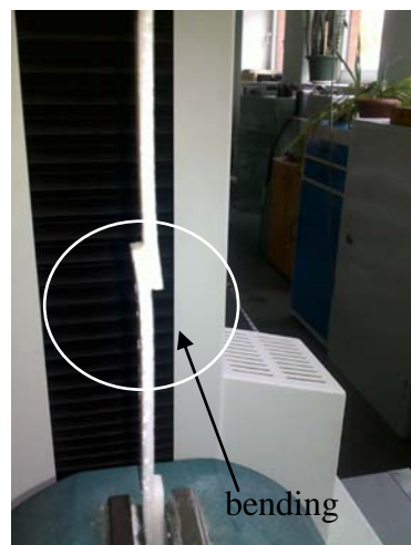
Fig. 7. Material bending before cracking
