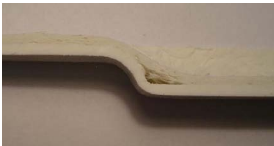
Fig.2. The sample of the defective adhesion
