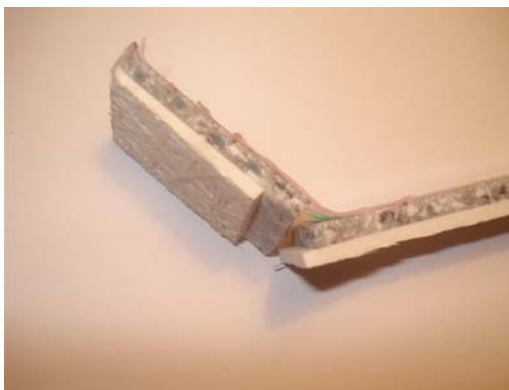
Fig. 4. The acrylic material break down
