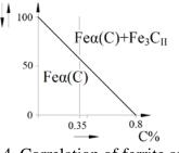
Fig.4. Correlation of ferrite and eutectic
