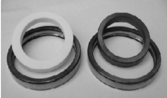
Fig. 1 Workpieces of technical ceramics SiSiC [5]
