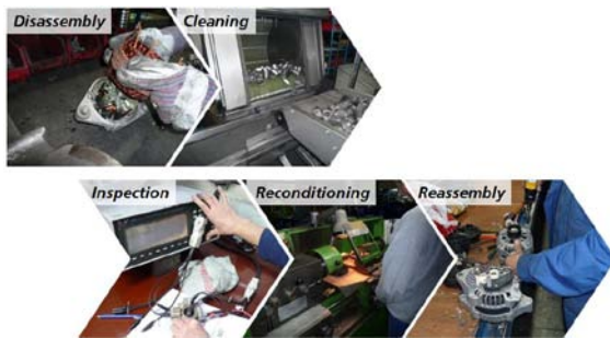
Fig. 2. Starters and alternators: Five steps of industrial remanufacturing
