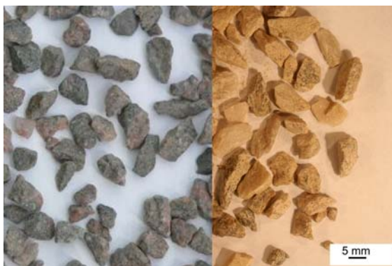
Fig. 7. Overall picture of abrasives: left side – granite gravel; right side – hard rock
