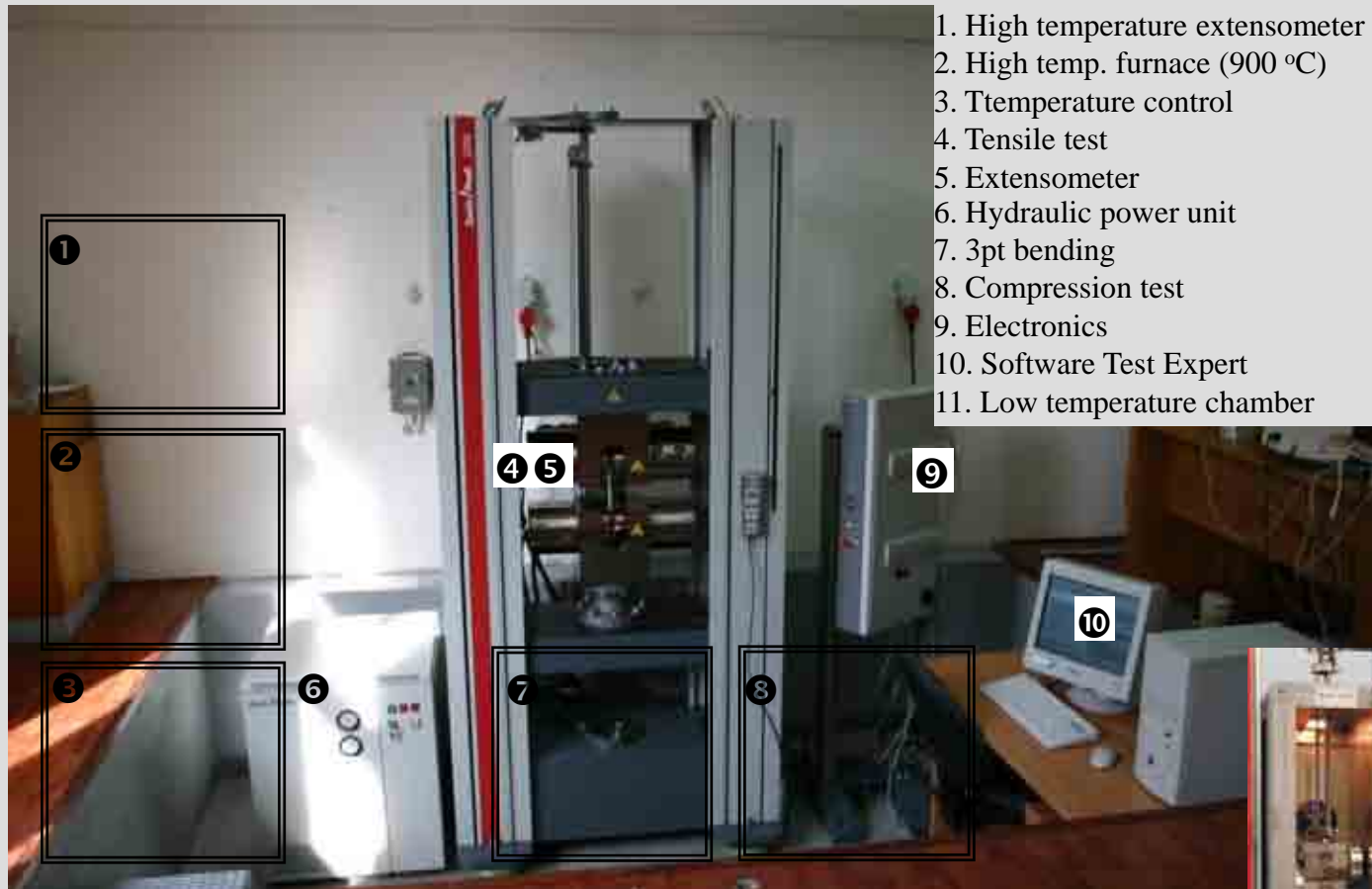
Testing system Zwick Z400E – 400 kN
