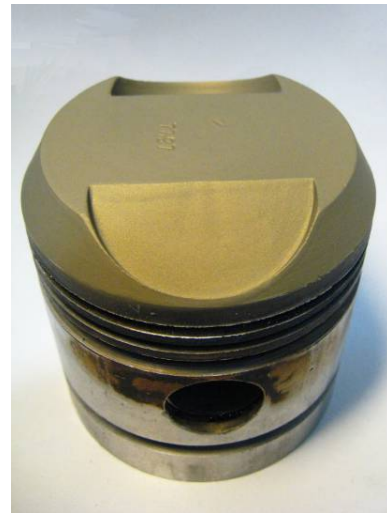
Fig.6. Piston coated with V 136.
