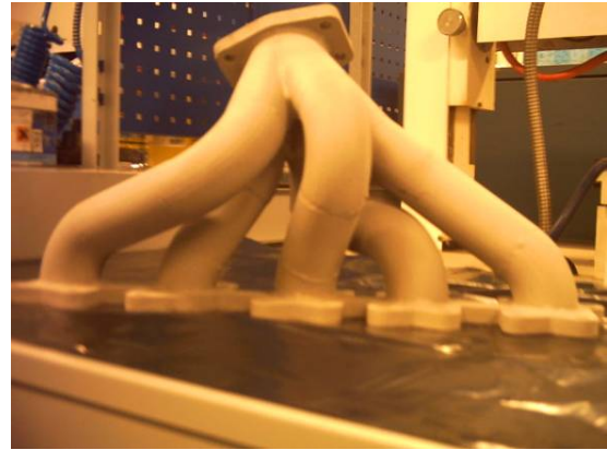
Fig.5. Barrier coating on exhaust collector.
