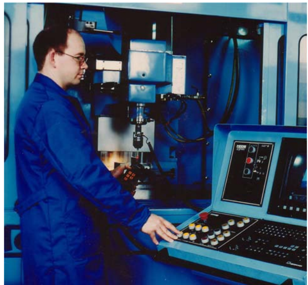
Fig. 1. The vertical-type machining centre Modig MD 7200 in the laboratory of HUT.
