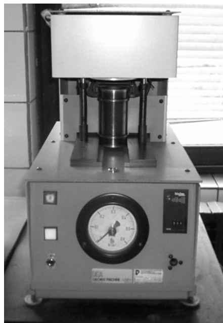
Fig. 3.2 Apparatus for measuring of wet tensile strength+ GF + type PZN
