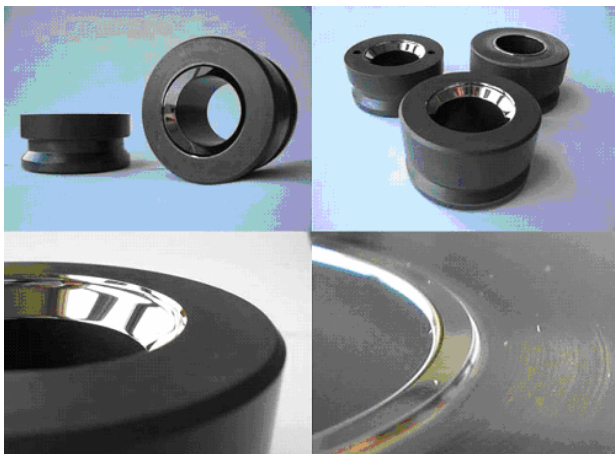
Figure 9 Ultra precisely machined crimping tool inserts for PVD WC/C coating
