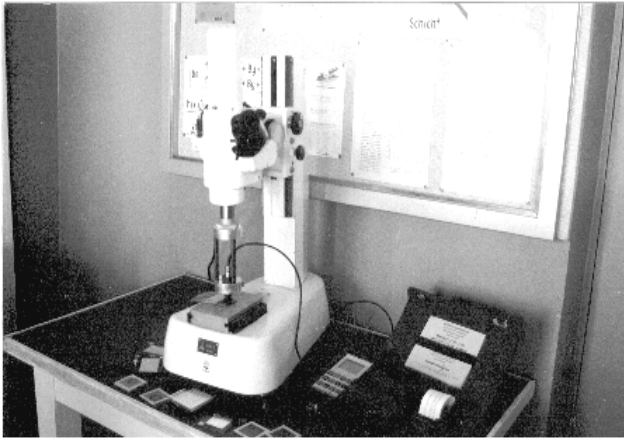
Fig. 4. Coating thickness standard measuring instrument
