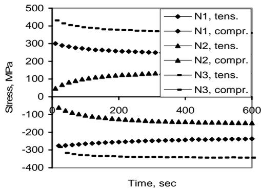
Fig. 3. Effect of HCF (by 1% of axial deformation) on deformation hardening-softening of copper by tension and compression: N1-cold-drawn, N2-recrystallized, N3-nanostructure state.
