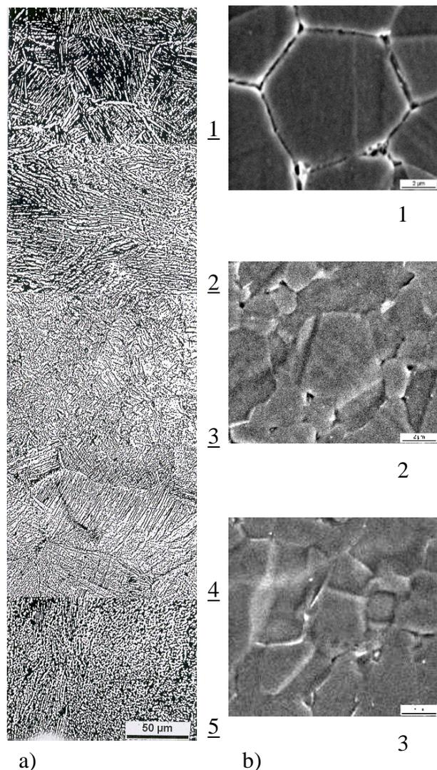
Fig. 2. Microstructure transformation by EUF is shown. Ti-alloy (a-column), and Ni-based superalloys (b-column).
