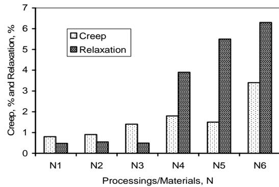
Fig. 4. Creep and Relaxation of materials vs. manufacturing technologies: N1-EUF processed Ni-based superalloy, N2-Extruded and die-forged Ni-based superalloy, N3-Cast monocrystalline Ni-based superalloy, N4-Cold-drawn copper, N5-Recrystallized copper, and N6- ECAP processed nanocrystalline copper.
