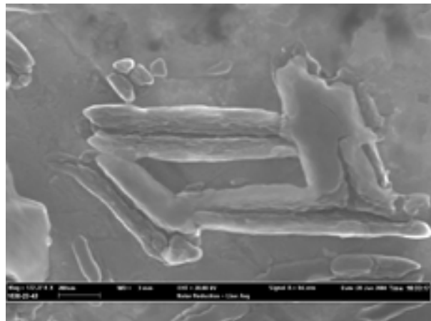
Fig. 2. On SEM picture of composite the chemical compounds, which were formed during high temperature heat treatment is shown. They have influence on mechanical properties relaxation, and spontaneous disintegration of composite.
