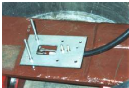
Fig. 2. High voltage discharge element and hard experimental cleaning surface.
