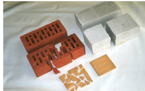
Fig. 12. Three cases of efficiency of high voltage discharge system: - demolish of porous brick; - demolish of full brick; - demolish of thin ceramics.
