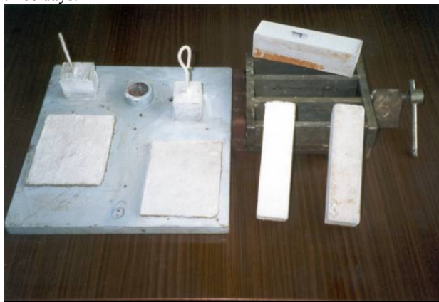
Fig. 4. Three kinds of experimental specimens: - cubic; - thin plane; - beam. All was made by concrete structure with different proportions of components.
