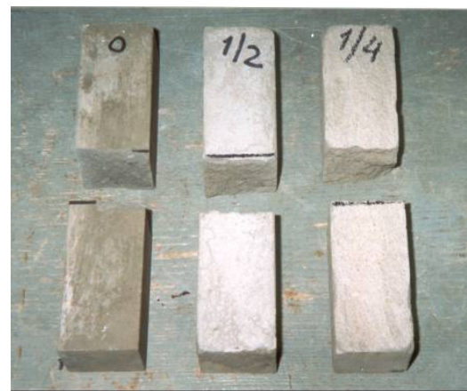
Fig. 7. Different bending experiments with different hardness of specimens to find crash strength. Crash fracture is in the middle of specimen.
