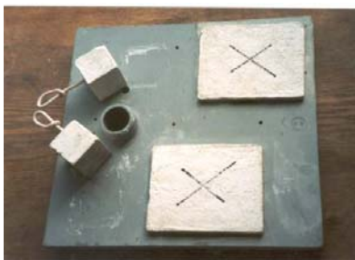
Fig. 5. Different tensile experiments for specimens to find negative boundary stresses (left side).
