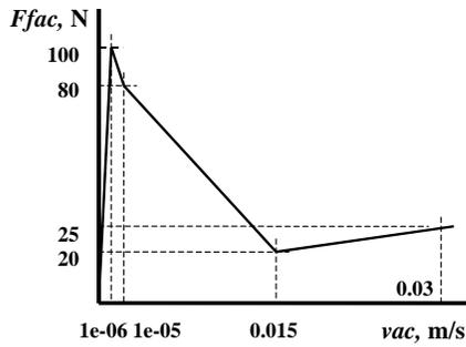
Fig.10. Friction force of an actuator  $F_{fac}$  as function of the actuator velocity  $vac$ .
