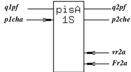
Fig.2. Multi-pole model **pisA1S** of piston, where
