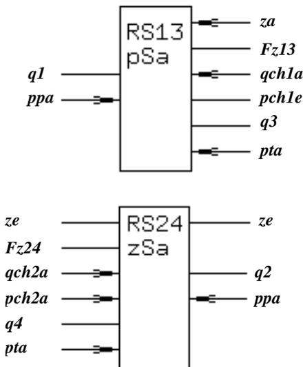
Fig. 1. Multi-pole models **RS13pSa** and **RS24zSa** of servo-valve slot pairs.
