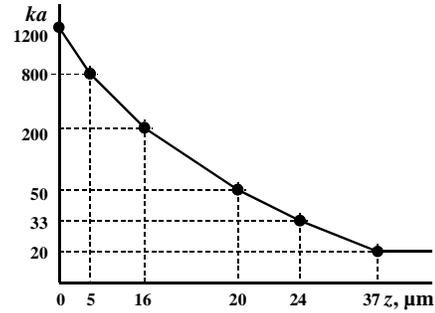
Fig.12. Amplification coefficient  $ka$  of regulator as function of the servo-valve position  $z$ .
