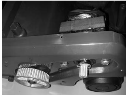
Figure 2. Power transmission system (with belt removed for clarity)
