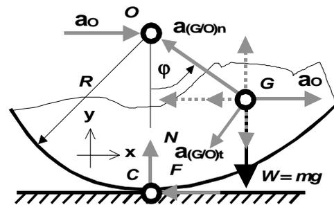
Fig. 1. Vectors on noncentroidal body when rolling starts
