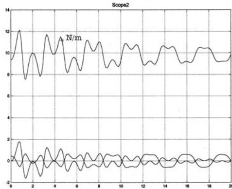
Fig. 6. Normal reaction and its component behaviour during free oscillations of the body
