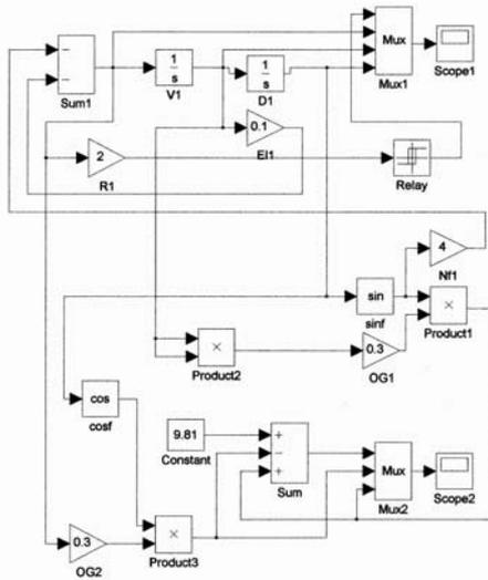
Fig. 4. Simulation block diagram for analysing free oscillations
