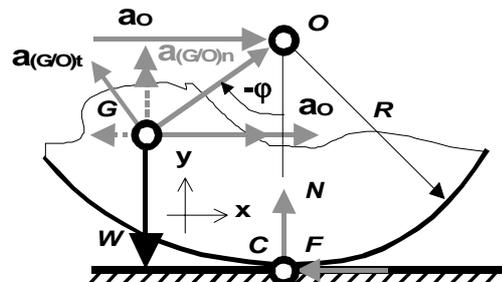
Fig. 2. Vectors of noncentroidal body when sliding starts
