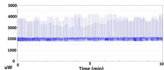
Fig. 6. Power usage of controlling circuit board at -24 °C temperature.
