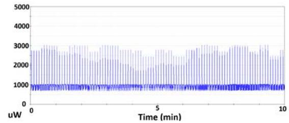
Fig. 4. Power usage of controlling circuit board at +8 °C temperature.
