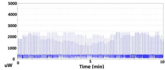
Fig. 3. Power usage of controlling circuit board at +24 °C temperature.
