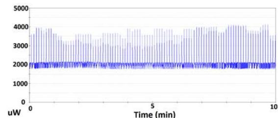
Fig. 5. Power usage of controlling circuit board at +2 °C temperature.
