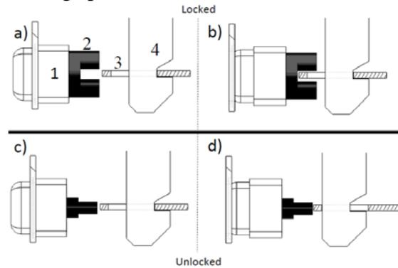
Fig. 1. Illustrations of the lock in different states. Figure a) show the lock in closed state at rest and in figure b) button (1) is pressed while lock is still in closed state. In figure c) lock is in open state when the button is not yet pressed and in figure d) button is pressed while lock is in open state.
