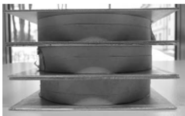
Fig. 4. Reinforced testing specimen: block with 3 rigid bonded rubber hollow cylinder
