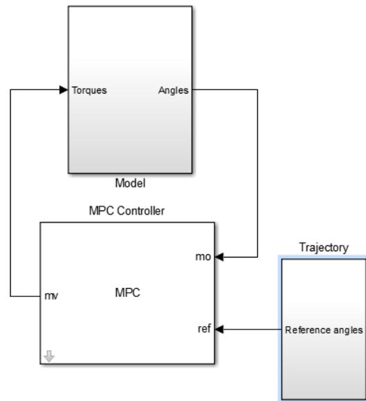
Fig.2 Matlab/Simulink scheme
