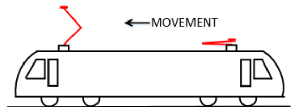
Fig. 1. Train with backward position of pantograph – Position P1
